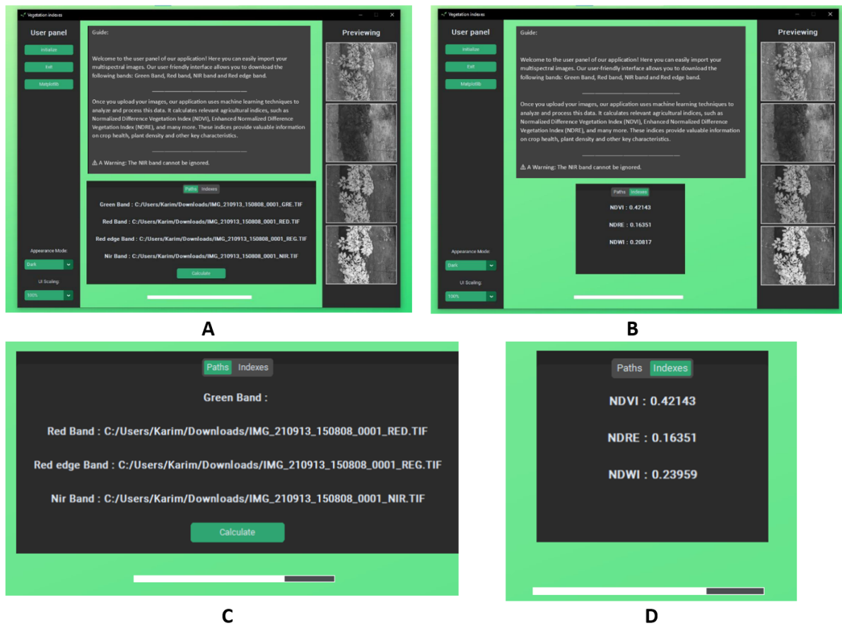
Figure 15. Application User Interface : (A) Image upload, (B) Indices calculation, (C) Ignoring the Green Band, (D) Indices prediction
