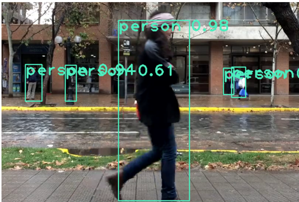
Figure 8. YOLO algorithm results for human detection.
