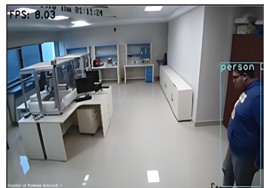
7b) Human detection results after stream undistorting
