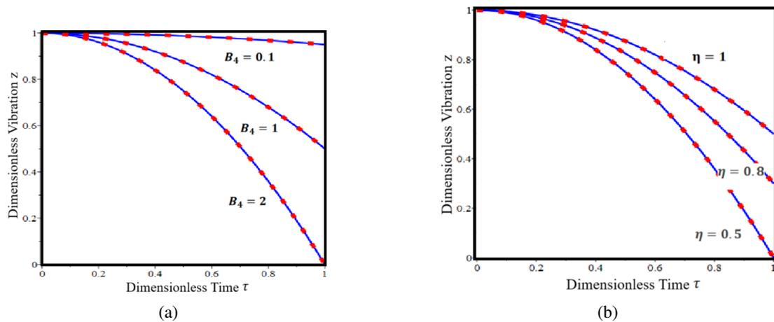
Figure 4. Figure showing the dimensionless vibration response  $z(\tau)$  versus dimensionless time  $\tau$  for various parameter combinations  $\alpha = 2, \beta = 1, \eta = 0.5, B_1 = 2, B_2 = 1, B_3 = 1, B_4 = 0.1, X_1 = 1, X_2 = 1, X_3 = 1$  as calculated as Eq.(13)
