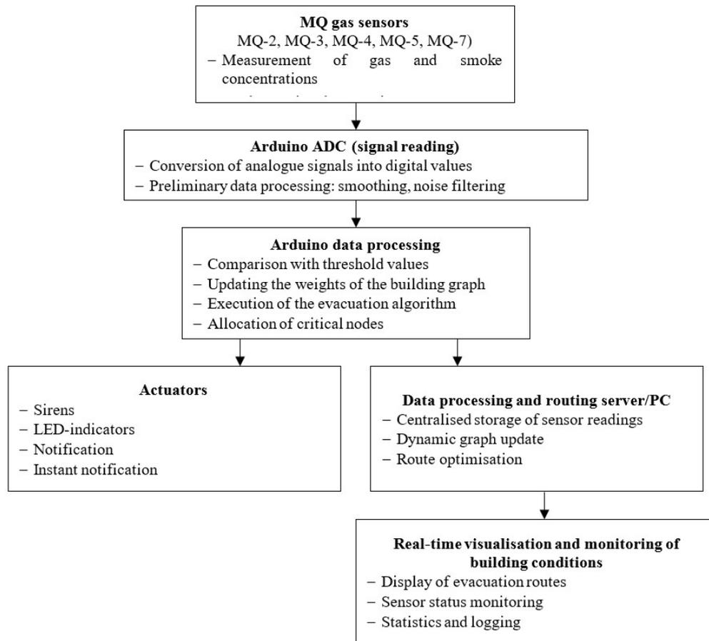
Figure 1. Integrated system data processing conveyor.
