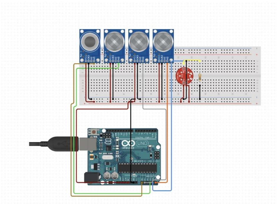
Figure 2. Diagram for connecting gas sensors to Arduino.
